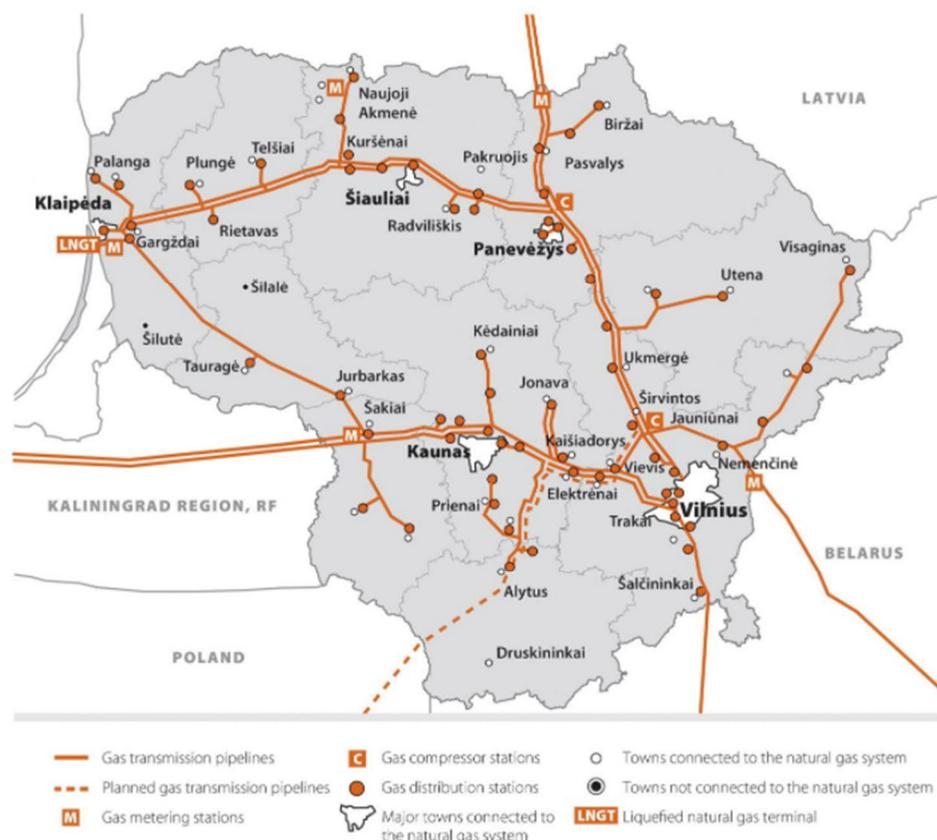
Figure A3-1.1: Overview of the Natural Gas Transmission System in Lithuania
